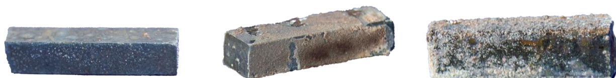
84MoSi 2 -10SiC-6ZrB 2 , 1820°C 33MoSi 2 -33SiC-33ZrB 2 , 1830°C 20MoSi 2 -60SiC-20ZrB 2 , 1750°C
